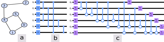
Fig. 2: An example graph for n = 6 (a), its encoding circuit (b) and the variational circuit (c). (b) and (c) are connected. Measurement circuits are assumed immediately after (c).
